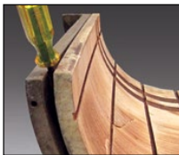
AFTER: Reline with Duramax® engineered polymer compound.
