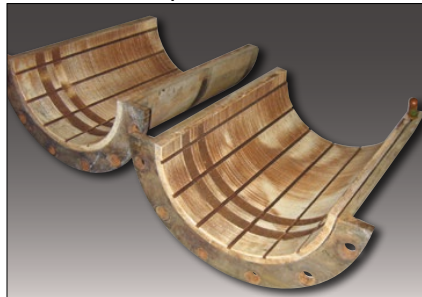
Bearing's surface embedded with abrasives.
