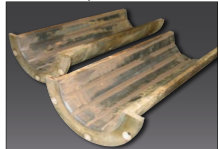
BEFORE: Duramax® Cutless® bearing after 16 years in service.
