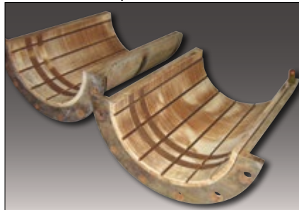
Bearing's surface embedded with abrasives. Polyurethane material de-bonded from housing.
